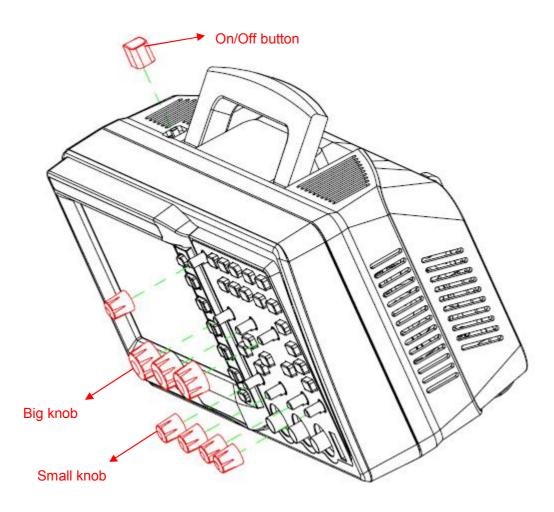
Figure 5-1 Removing the Front -Panel Knobs
