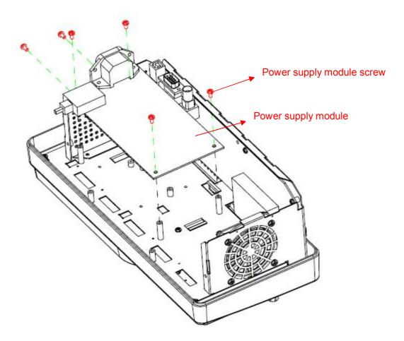
Figure 5-5 Removing the power supply module
