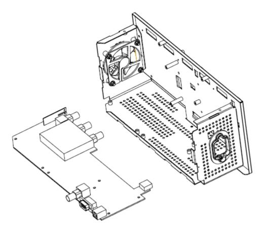
Figure 5-8 Removing the main board module
