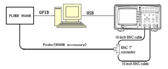
Figure 4-1 Connecting the adjusting devices
