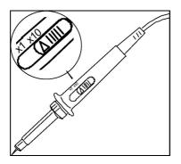
Figure 2-2 Set probe attenuation switch
