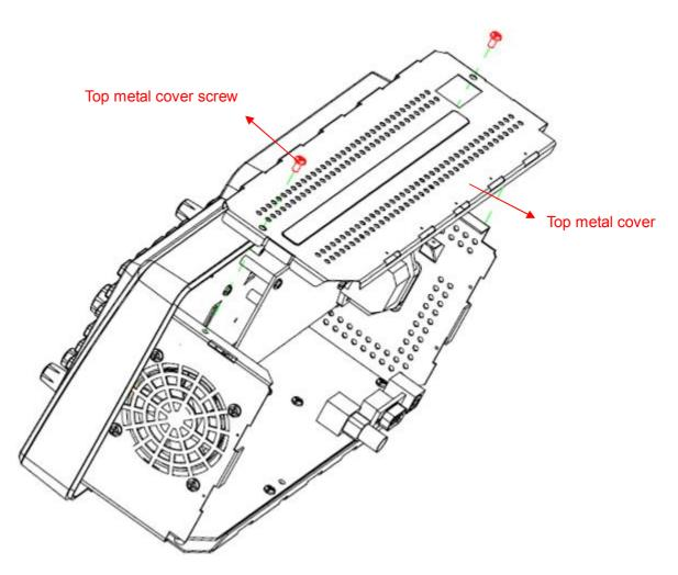
Figure 5-4 Removing the top metal cover
