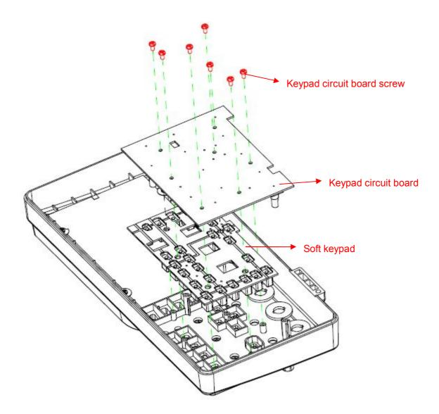
Figure 5-11 Removing the Keypad Module
