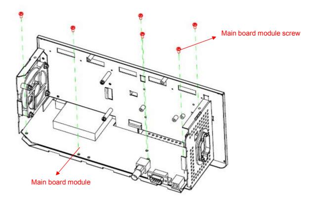
Figure 5-7 Removing the main board module
