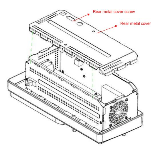
Figure 5-3 Removing the rear metal cover
