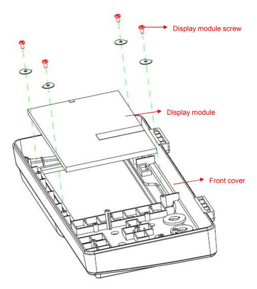
Figure 5-10 Removing the Display Module
