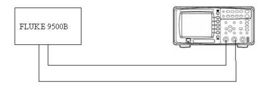
Picture 3-1 Connecting test instruments
