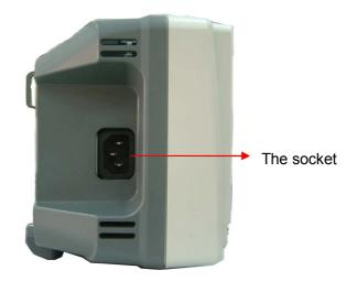
Figure 2-1 Connect power line
