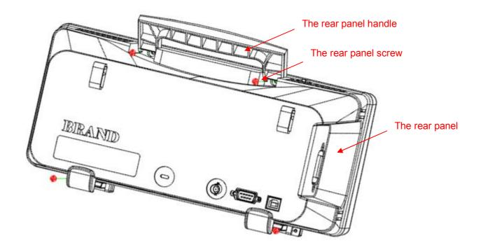
Figure 5-2 Removing the rear panel
