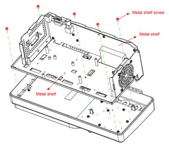
Figure 5-6 Removing the Metal Shelf
