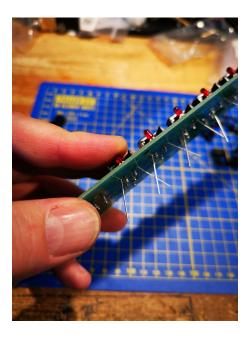
Now you can place the actuator with LED onto the tact switch, make sure the actuator is fitted flush and splay the LED legs to hold it in place. Once you have fitted them all, solder and clip the legs.
