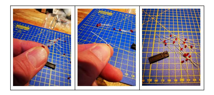
Now we must prepare the leds, first bend 16 of them out like so. It's easy if you hold the tip and splay each side one at a time as in the pictures.
