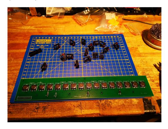
First place the tact switches, it's a good idea to only solder the opposite pins of each switch and then check everything is sitting well and aligned correctly. It'll be a lot easier to heat a leg and fix any mistake now than later on. If they all look good, solder the remaining legs.
