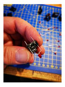
Now you can place the LEDs into the actuators, the long leg of the led should be on the right.
