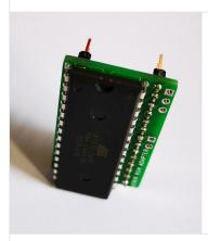
Test fit the eprom, as with all new IC's you will need to straighten the legs a little. If you dont have an IC pin straightening tool you can straighten pins for insertion by "rolling" the chip on a flat surface, bending one side of pins together slightly at a time and not further than the 90 degrees needed.
