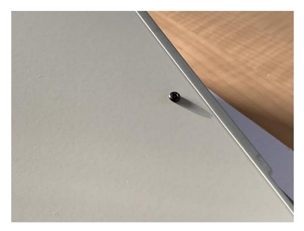
Now everything should be ready and you can attach the supplied adhesive feet, or other device feet with M3 screw connections, if you have any.
