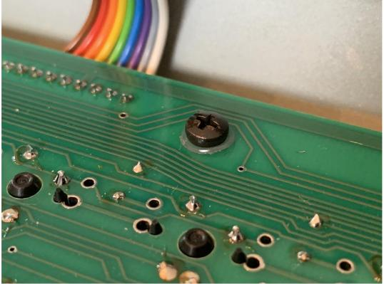
Connect the cables between the sequencer board, audio board, etc. and carefully place the audio board in the case. Screw the board with the M3 screws and the thick plastic washers. I used my beta board for this guide, so don't be surprised how it looks! Again, before tightening the screws, make sure that the shafts of the potentiometers are well aligned!
