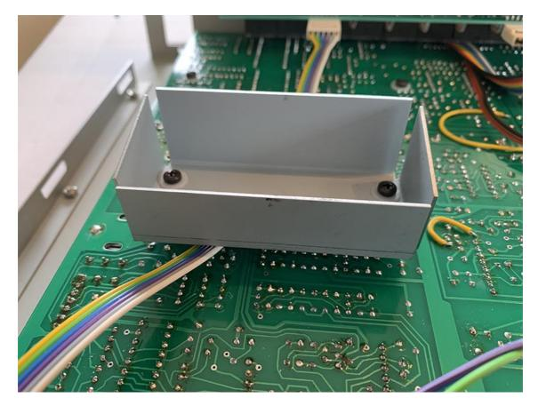
Now you can install the base plate with 6x M3 screws. Screw in only lightly at first, check the alignment of the plate and then tighten.
