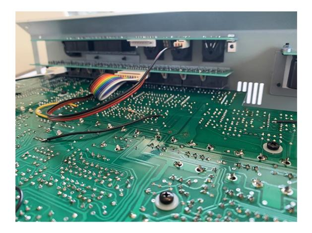
The two short nylon spacers are screwed in on the left side. These will hold the battery compartment.
