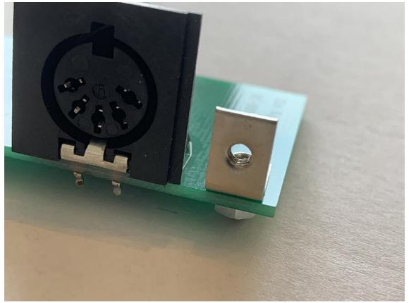
Please make sure that the Z-bracket is parallel to the PCB after screwing, otherwise the audio and MIDI sockets will sit crooked behind the case holes.
