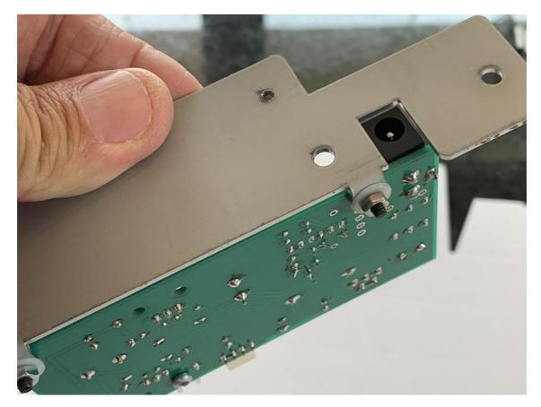
Next we mount the metal brackets on the MIDI board. For this we need the short Z-bracket and the small L-bracket with the M3 hole.
