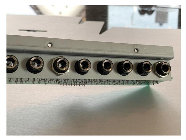
6x M3 screws with washers are required for mounting the audio and MIDI circuit board on the rear of the case.
