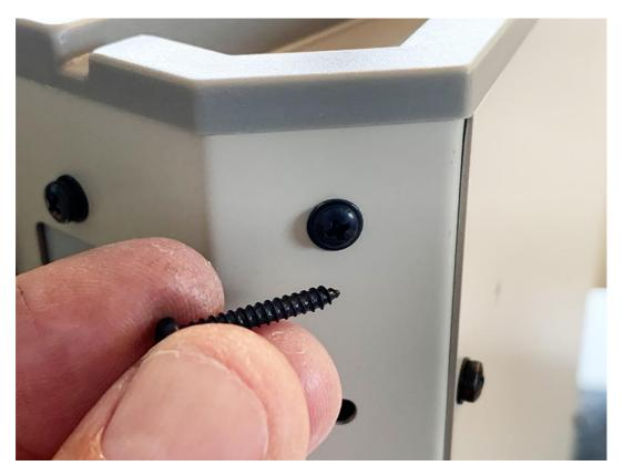
Two screws are screwed in from the short slope and the other two from the base plate.
