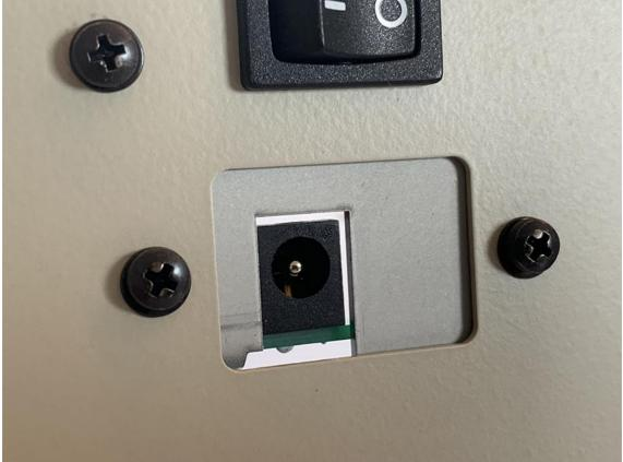
Now we come to the sequencer board. Carefully place the circuit board in the housing and screw it on. On the lower edge with 5x M3 screws and the thin plastic washers. On the upper edge one M3 screw in the middle and left and right with the 13mm nylon spacers.
