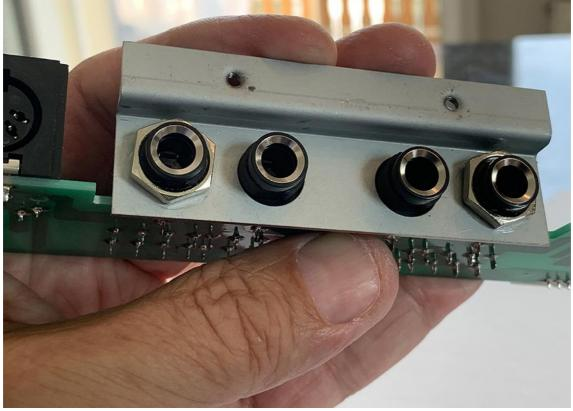
Attaching the M12x1 nuts is a bit fiddly, but it works. As can be seen in the photo, only two of the nuts are used, each on the outer sides. The small angle is attached to the side so that the side with the M3 thread protrudes upwards.
