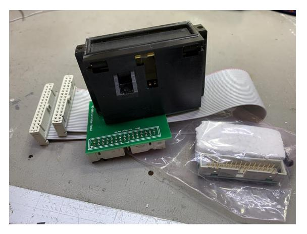
First, remove the protective foam from the HIF2C adapter PCB and check for bend or broken pins.
