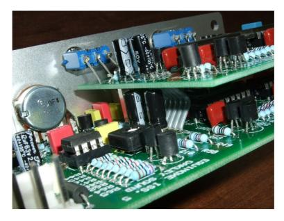
The view between the two boards. Low profile electrolytic capacitors would probably have been better in this case as the two lower ones nearly touch the underside of the Deep Equinoxe board.
