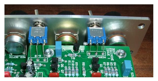
The switches are simply wired to the Deep Equinoxe board with stiff solid core wire although you can use multistrand hook up wire if you like. The solid core wire is looped around each switch lug and soldered in place. I recommend that the wire has some slack to allow the boards to flex a little.
