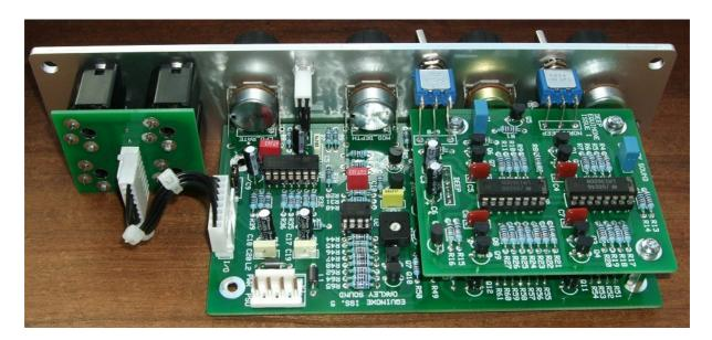
This is the issue 1 Oakley Deep Equinoxe module behind a natural finish Schaeffer panel. The Deep Equinoxe board is the smaller one mounted above the standard Equinoxe PCB. Note the use of the optional Sock4 socket board to facilitate the wiring up of the four sockets.
