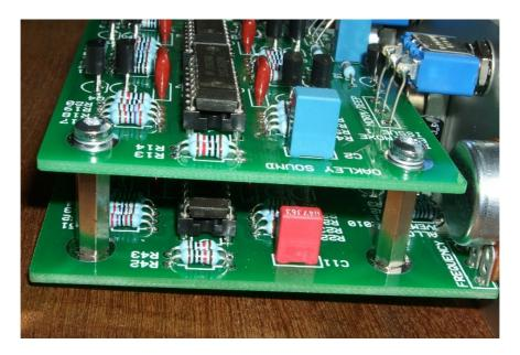
A view showing how the two boards are attached to one another..
