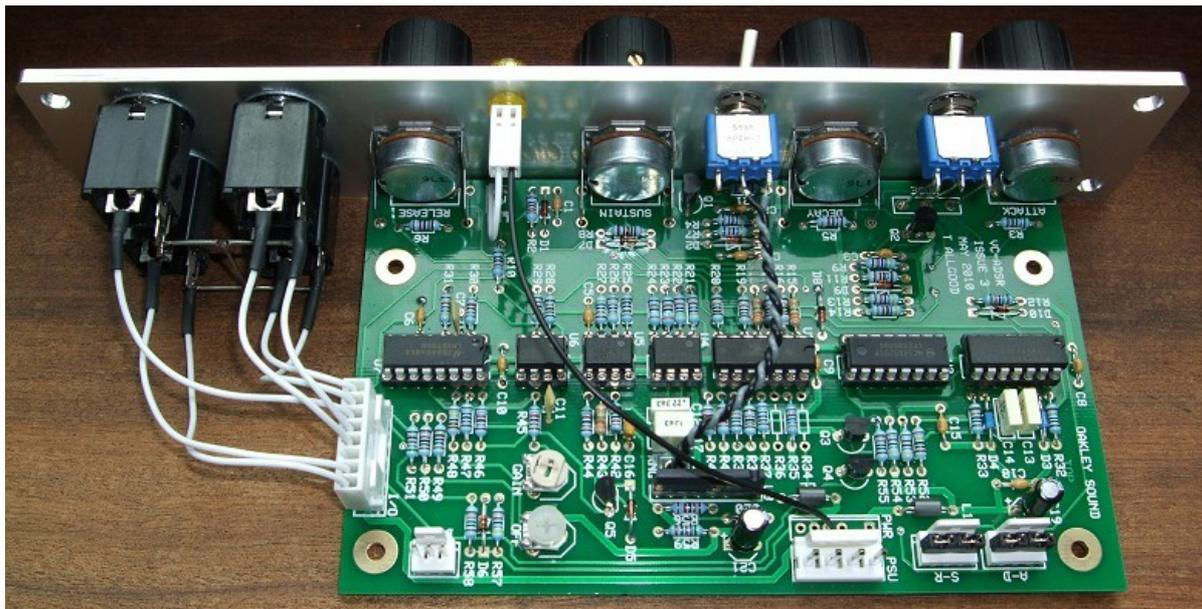
*This older style panel fitted to an issue 3 PCB has used hand wired sockets.*
