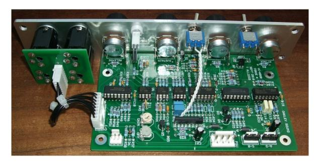
The issue 4 VC-ADSR/VCA board mounted behind a natural finish Schaeffer panel. Note the use of the optional Sock4 board to mount the jack sockets. Note also the two 0.1" KK headers on the lower right. These headers can be attached to the 1U Upgrade module to allow for full voltage control of the modules four parameters.
