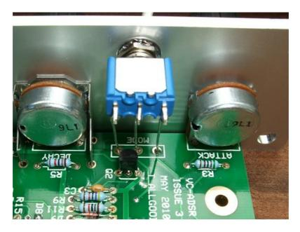
*The solid core wire is looped around each switch lug and soldered in place. The switch needs to be in its place and tightened before soldering the leads.*
