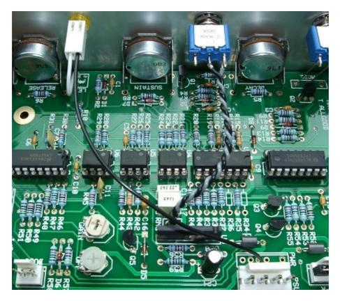
*Issue 3: The black wire is the cathode connection and carries the ground connection to the LED. Notice I have used a Molex KK 0.1" header to neatly attach the connections to the LED.*
