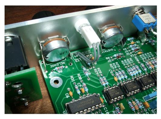
Using Molex KK 0.1" housings and crimps makes connecting to the LED very simple. The LED clip used here is a 5mm low profile clear type with a white plastic securing ring. The actual LED is a green LED in a water clear package. This is an issue 4 board, the earlier issue 3 boards require the cathode connection to be taken back to the power supply header – see later for more details.
