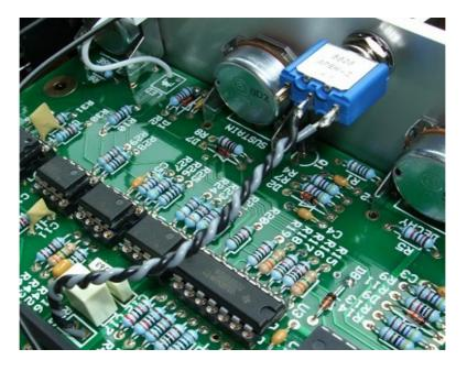
It is the top two lugs of the switch that connect to the two pads of RNG.
