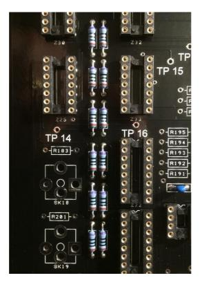
7. Add the remaining resistors. Note the three (larger)  $\frac{1}{2}$ -Watt resistors for the LED chains (R81, R106 and R242).
