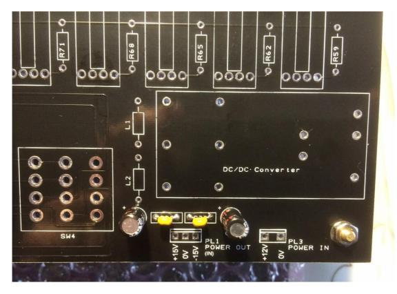
4. Add the remaining capacitors. Note the location of the film-type (grey) caps and the X7R (yellow) type in the photo
