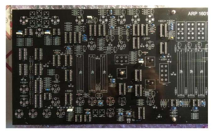
5. Add the eight trimmers. Leave approx at half-way setting on each. Note there is some doubt whether two of them (R217 and R218) should be 1k or 2.5k. The original schematic shows 1k and the parts list 2.5k. From the final position after tuning, 1k seems to be the more appropriate value. Both are in the BOM should you wish to experiment.
