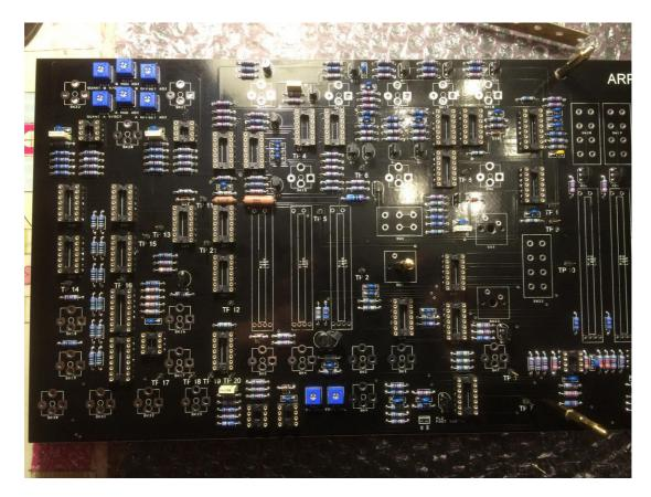
Nevertheless, Q4 and Q5 need to be pushed together for thermal coupling, and held with a cable tie or similar
