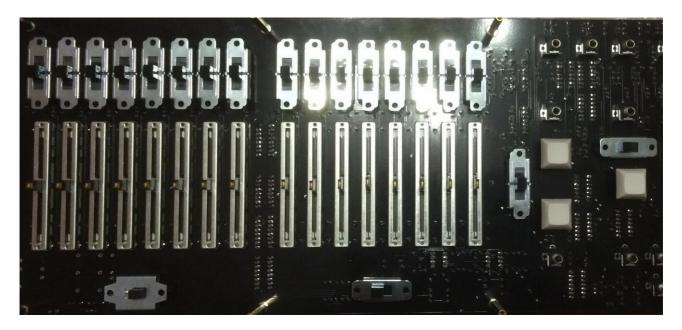
14. Fit the three headers, the 21 test point pins (from the snap-off 0.1" header strip), the DC/DC converter and two ferrite beads on wire links for L1 and L2. The three-pin power header (PL1) then becomes an Aux supply for anything else you may wish to power, up to the rating of the DC/DC converter. The 1601 draws only circa 64mA on the +15V rail and 34mA on the -15V rail so there's plenty to spare for other uses should you wish.
