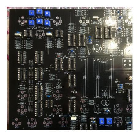
6. Add the twelve 100R precision resistors which make up the equivalent of the quantizer resistor pack Z20 in the original design.
