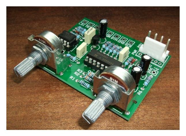
The issue 6 Little-LFO board fully populated. The MTA156 header has been fitted to this one allowing it to connect to the Oakley/MOTM and Fractional Rack modular systems. The pots used here are the ones with a short 6mm knurled shaft.
