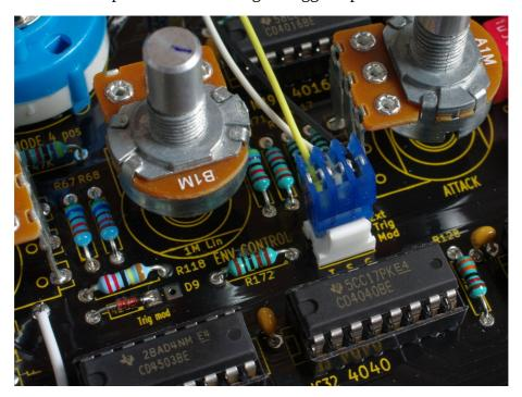
This is based around D9 and R172, and the Ext Trig Mod header used to connect a switched jack socket. R172 is added protection for larger trigger voltages.
