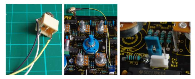
For testing, or if you do not wish to use the external trigger mod immediately, simply jumper the T and S pins on the header as above.
