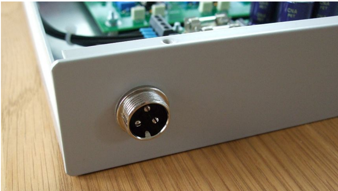
The three way power socket that will fit the Yamaha PA20 power supply.
