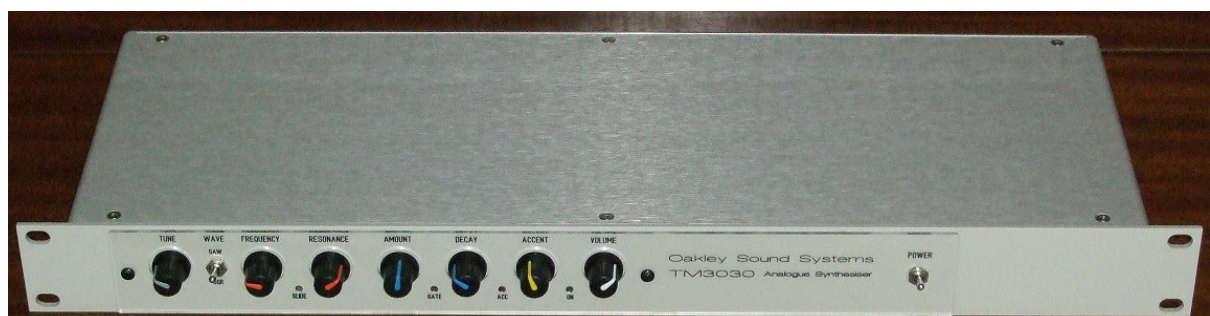
The second issue 1 TM3030 I built. This one has been built into a 19" rack from Holt Broadcast. The front panel legending is achieved with a thin perspex overlay, cut and engraved by Schaeffer in Germany.
