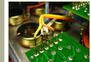
Run these wires to pads x and y on the meter board. The polarity is actually unimportant so if you happen to switch x and y around you'll never notice it, operationally. But don't make it a habit to neglect this sort of detail as eventually it will turn around and bite you...
