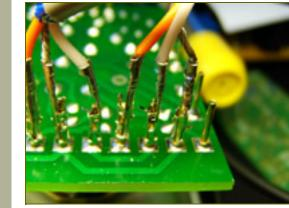
Wire the other end of the output pot cable to the three output pot pads on the ratio board which are right next to pads 15, 16 and 17. Note the arrangement carefully shield on the outside (with the trace running to the other shield wire), wiper terminal in the middle.
