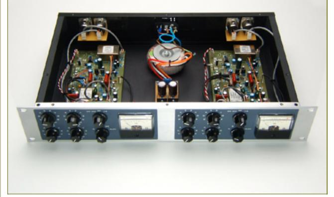
Wiring the 1176LN Clone - Rotary Version
