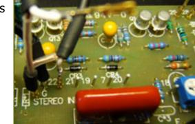
Leave the other cable unconnected for a while. There are lots of pads in between and it is easier to access them if you don't have the other wire hooked up and potentially blocking your view.
