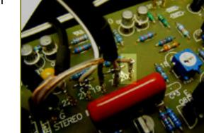
Finally, to finish this row of pads, solder the other end of the wire from pad 20 of the main board to pad 20 on the ratio board.
