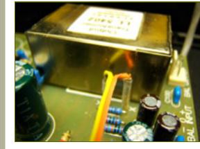
Now grab the output signal from pads x and y. These pads are located near the output transformer. The signal from these pads will show the output level of
