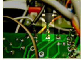
Solder the wire that came from pad 7 of the main board to pad 7 of the ratio board.
