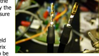
Put a length of shrink tubing over the exposed shield leaving only the inner wire, or in this case the matrix socket, sticking out. Only the inner wire is going to be connected at the other end.
