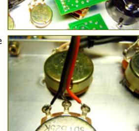
The attack pot gets connected to the ratio board too. Note carefully where each of the wires goes - wiper in the middle, counter-clockwise leg (the one that the wiper comes to rest on when the pot is viewed from the front and turned to the furthest counter-clockwise point) nearest the edge of the board.
