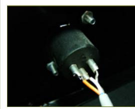
Now wire the output jack with two-conductor shielded cable. Pay close attention to the markings on the XLR housing - terminal 2 is +, terminal 3 is - and 1 is neutral or shield. Note that the output jack terminals (male XLR) are the mirror image of the input jack terminals (female XLR).
