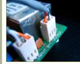
The other end of the two-conductor cable attaches to the main board at the output pads. These pads are located right near the output transformer. Please note that if you are using Jakob's rev 7 boards the pad designations are reversed, that is, the pads go - 0 + leftto right. My boards go + 0 - left to right, the opposite of the input pads.
