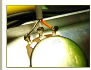
Using two conductor shielded cable, wire the output pot as shown. Use any colors you want, just make sure they correspond to the correct points on the opposite end of the cable...
