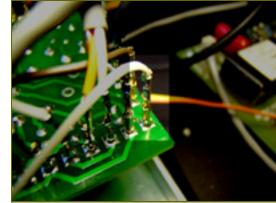
Wire the other end to pad 4 on the ratio board, right next to where the output pot wires go.
