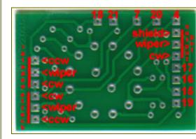
Because all of my shots of the ratio and meter rotary switch boards are shown with the printed circuit boards upside-down, I've made up some scans to give an overview of where the connections are made. Of course, if you have my boards in hand, you can just flip them over to see the silkscreen designations but these pictures should help you out if you are doing a homeetch or are using other boards that don't have all the designations. (Note: the ratio board, like most of the
