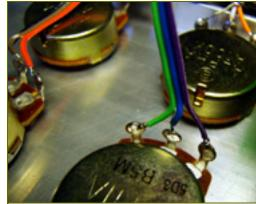
Wire the release pot (4.7 or 5M) in a similar manner to the attack pot using unshielded wire.
