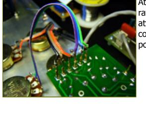
Attach the other end of the release pot wires to the ratio board. Note that they go in reverse order of the attack pot wires. Look at the violet wire which orresponds to the clockwise rotation of the potentiometer. The wiper goes in the middle again.
