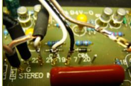
The wire from pad 19 on the main board goes to pad 19 of the ratio board, right beside the shielded cable that ran from the main board pads 15,16 and 17.
