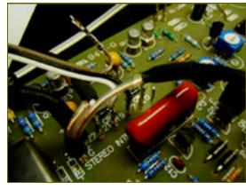
Now put that other piece of shielded wire you left a while back through to pad 7 on the main board.
