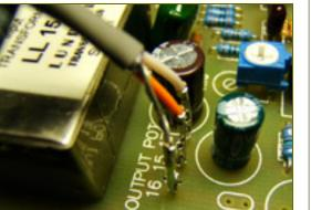
Wire a length of two conductor shielded cable to the points marked 16 15 17 on the main circuit board. Note that the outer shield is connected to terminal 16.
