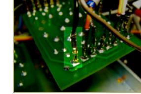
Solder the wire from pad 21 of the main board to pad 21 of the ratio board.
