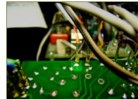
The other end of the wire from pad 18 on the main board goes to pad 18 of the ratio board.
