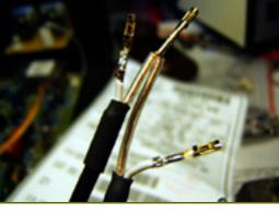
Put a little shrink tubing over the shield wires and some larger shrink tubing over the gap where the outer insulation was stripped back. The two shield wires are different lengths for a reason - one of the cables is going to connect to pad 22 on the main board and the other is eventually going to connect to pad 7.
