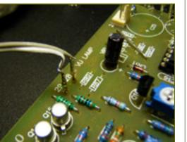
Solder one wire to each of these pads. They do not need to be shielded. You can use ribbon cable as I did or just twist a pair of stranded wire together.
