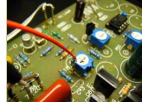
Solder a plain wire to pad 18 on the main board. Note that there are two holes near the "18" designation. If you use a large trimpot, you may need to use the hole *above* the "18".
