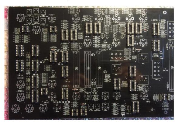
3. Add the power supply smoothing capacitors. Note orientation of the two electrolytics, and the two 100nF X7R types. For Rev 2 PCBs, L3 and C40 are fitted by PL3.
