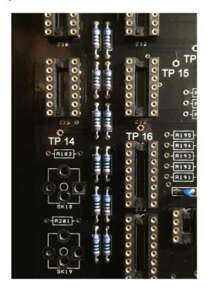
7. Add the remaining resistors. Note the three (larger) ½-Watt resistors for the LED chains (R81, R106 and R242). I have substituted the oversized ceramic body resistors in recent versions of the BOM – they should fit perfectly well now.
