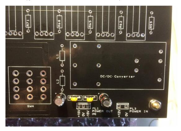
4. Add the remaining capacitors. Note the location of the film-type (grey) caps and the X7R (yellow) type in the photo. Mod: Instead of a 10nF C0G/NP0 capacitor for C5, use a 33nF or 39nF, whichever is available. There will be another capacitor to add later.
