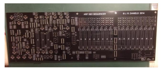
2. Add the five diodes. Check orientation – black line on diode to white line on PCB (pointing to the right on all but D2 which is to the left). Note that the diode numbering is not D1 to D5 inclusive, as most of the diodes are LEDs and form part of all 19 sliders.
