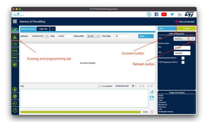
7. Press the connect button and go to the Erase and Programming tab:
