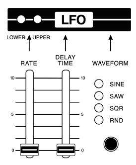
ISE-NIN has a very simple main Low Frequency Oscillator (LFO), however it can produce some advanced tones when routed separately to LOWER and UPPER sections in a Preset. LFO works identically for LOWER and UPPER sections.
