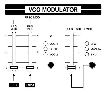
This section sets the amounts which the various modulation sources are applied to the pitch of VCOs 1 and 2: This section also controls modulator amounts to vary the width of PULSE when selected in either or both VCOs.
