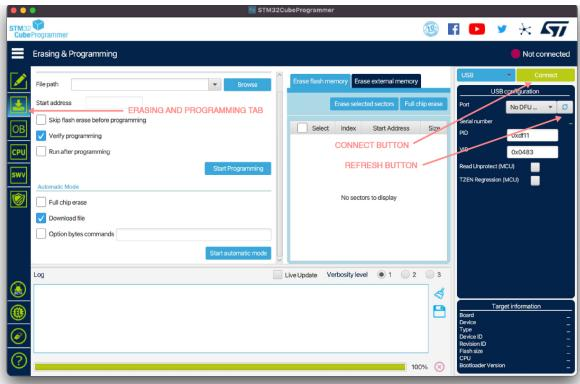
7. Press the connect button and go to the Erase and Programming tab:
