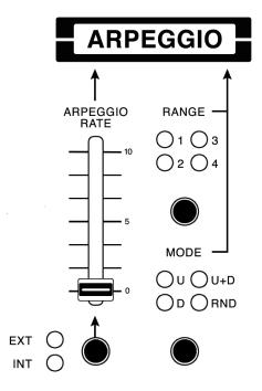
ISE-NIN's arpeggiator section allows for automatically playing and shifting notes harmonically in real time. This can be useful for improvising during a performance or for inspiring ideas while composing.
