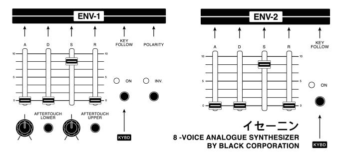
ISE-NIN features two envelope generators that are used to shape the sound over time. These envelope generators are typically labeled as Envelope 1 (ENV-1) and Envelope 2 (ENV-2).
