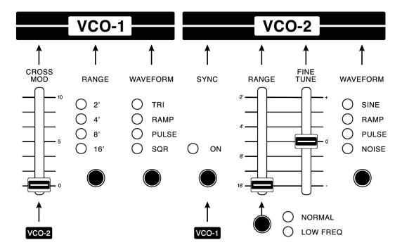
\ISE-NIN has two independent Voltage Controlled Oscillators (VCOs) per voice which are the main sound source of the synthesizer. They can be used together to create a wide range of tones and timbres.
