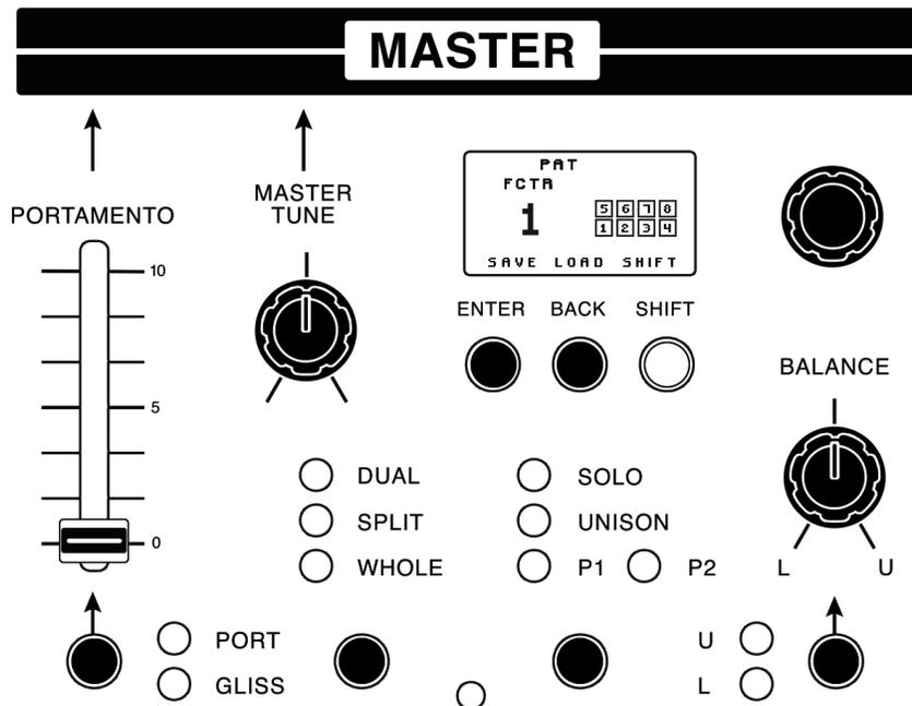
The DISPLAY along with the ENTER, BACK, SHIFT buttons and ENCODER knob navigate through the SETTINGS menu. ENTER selects a menu item or executes the selected function. BACK exits a menu or cancels a function. SHIFT accesses secondary functions as well as allows for some alternative adjustments of the sliders and knobs. The ENCODER is used to select presets, saved layers, and menu items. It can also be pressed to act like the ENTER button or switch between PRESET and PANEL modes.
