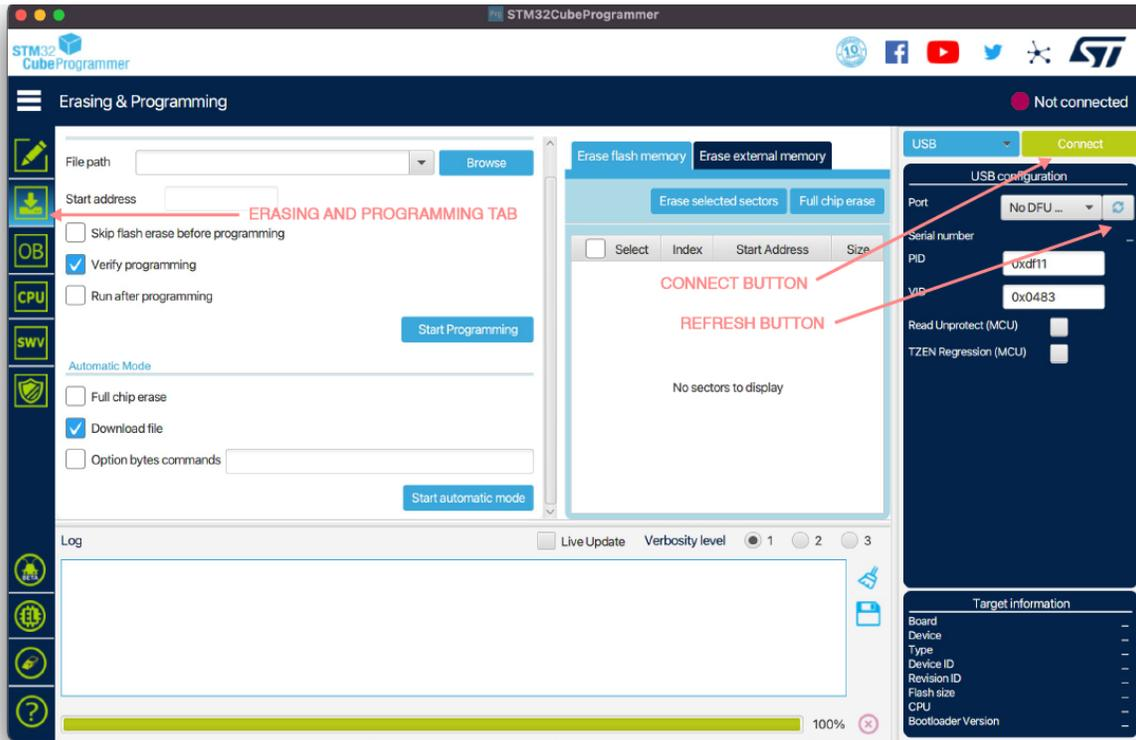
7. Press the connect button and go to the Erase and Programming tab:
