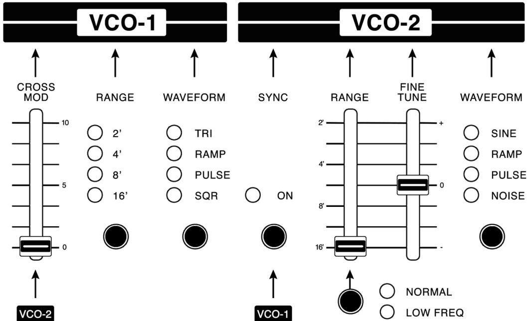
ISE-NIN has two independent Voltage Controlled Oscillators (VCOs) per voice which are the main sound source of the synthesizer. They can be used together to create a wide range of tones and timbres.
