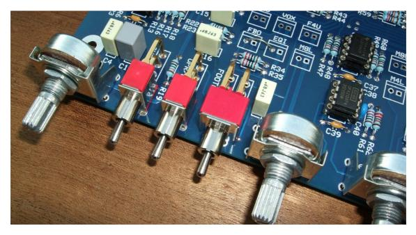
The three switches. These are made by Multicomp (part numbers 1MS1T2B4M7RE for the two SPDT and 1MD1T2B4M7RE for the single DPDT.)
