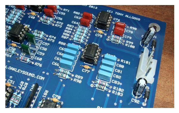
The power header on the HVM board. This is a 0.156" (3.96mm) Molex KK. This is similar to the MTA156 type connector that we normally use on our MOTM compatible modules but the two are not interchangeable. However, the KK is cheaper and only requires a cheap crimper to make the leads.
