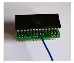
For the **Hi-Hats** eprom, **solder** a **flying** wire to the left square pad, (10cm will be more than enough.) and place a **jumper** between the circle pads as in the picture. Place the eprom on the main board **WITHOUT A SOCKET** and solder the other end of the flying wire to **pin 12 of IC73**. (do this after you have fitted IC73 and solder direct to the pin) This is needed to maintain compatibility with original Roland maskroms.
