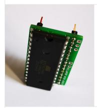
Test fit the eprom, as with all new IC's you will need to straighten the legs a little. If you dont have an IC pin straightening tool you can straighten pins for insertion by "rolling" the chip on a flat surface, bending one side of pins together slightly at a time and not further than the 90 degrees needed.
