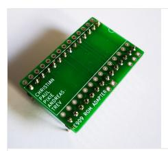
Solder the pin headers to the second and forth row of pins as shown.
