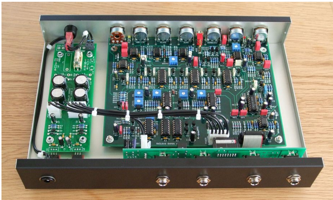
The rear panel connections are, from left to right, power input, delay output, mix output, CV input, and audio input.
